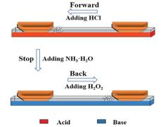
To improve the intelligence of smart devices and realize round-way smart motions, a smart device is fabricated with two types of actuators of magnesiumacid system and platinum-hydrogen-peroxide system at the opposite ends. Under acidic conditions, the magnesium reacts with acid to propel the device forward; changing to alkaline, the device stops motion; adding hydrogen peroxide, it moves back.
