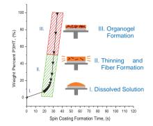
Poly(3-hexylthiophene) organogels offer exploitable electronic properties. These gels agglomerate into 3D percolating networks that span the active layer of a thin-film device. Novel spin-coating conditions that produce organogels in a rapid deposition process are discussed, including the interplay of kinetics and solution thermodynamics in organogel formation, control of the network size. and the correlation of structure to electronic properties.
