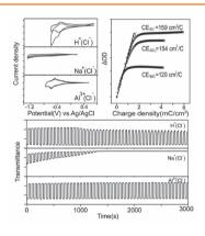
Using Al3+ as insertion ions in electrochromic applications allows for fast switching, high-contrast, and highly stable electrochromic behavior. It also makes it possible to overcome the existing problems encountered by the conventional insertion ions. The new, low-cost insertion ion is beneficial for the fabrication of more stable and economical electrochromic devices.
