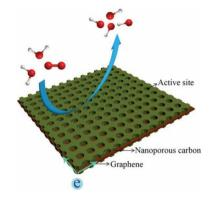
A zeolitic-imidazolate-framework nanocrystal layer-protected carbonization route is developed to prepare N-doped carbon/ graphene nano-sandwiches. These act as a highly active and stable nonprecious metal catalyst for oxygen reduction.
